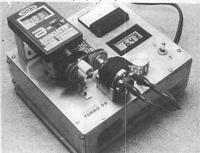
The Birtles Dyno. Motor under test drives a "slave" motor via Yokomo Dogfighter diff pulleys (mounted on a home-made boss) via a Dogfighter rear belt. "Loads" are applied by switching resistances across positive and negative slave motor brushes. Model Flight (SA) tachometer reads RPM, digital voltmeter reads voltage in (from 20 Amp power supply) and analogue amp meter measures current drawn by motor under test. This unit is home made but Mike O'Reilly of Model Flight (08) 293 3674 can supply something similar, but without the load feature, for around $200.
